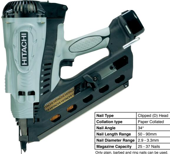
Only plain, barbed and ring nails can be used. The use of any other type of nail can result in tool malfunction.
