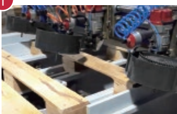
Automation: PN70PAL nailing decks to blocks
