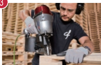
PN90 nailing bottom decks to pallet blocks
