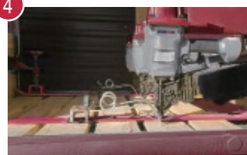
Automation: PN80PAL nailing decks to stringers
