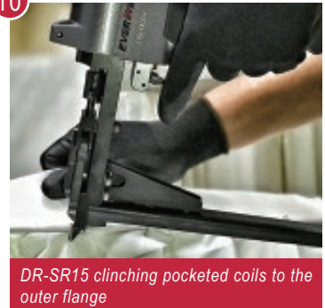
ECAR Stapling foundation spring to flat members
