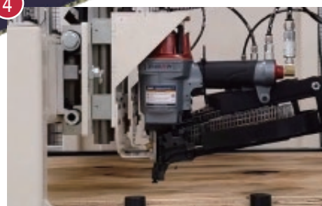
Automation: PN80PAL-JM at a sheathing station
