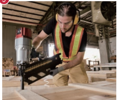
FSN160 securing deck boards to pallet jacks on a machinery crate
